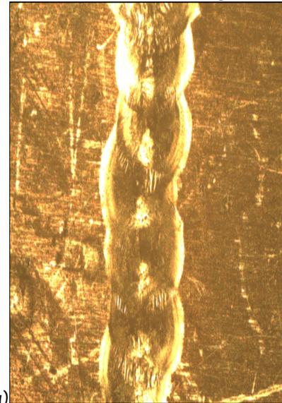
Figure 10. Spot laser welding of: a) wires  $\varnothing 0,5\text{mm}$  and b) strips from gold 585 alloy. ( $\text{Nd}^{3+}$ :YAG laser)
