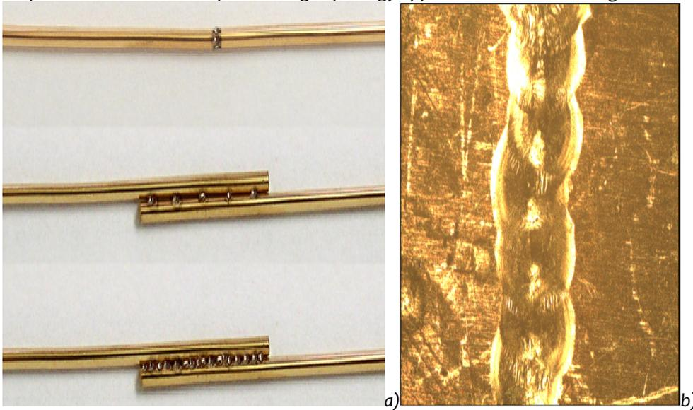
Figure 10. Spot laser welding of: a) wires  $\varnothing 0,5\text{mm}$  and b) strips from gold 585 alloy. ( $\text{Nd}^{3+}:\text{YAG}$  laser)
