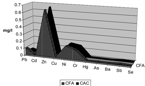
Figure 3. Results of leaching test performed on CFA and CAC samples
