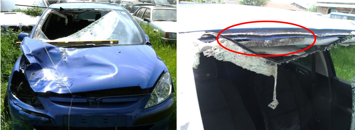
Figure 1. Photos of the front of the car (left) and of the part which produced the severance of the body of the pedestrian (the latter marked with red line in the photo on the right)
