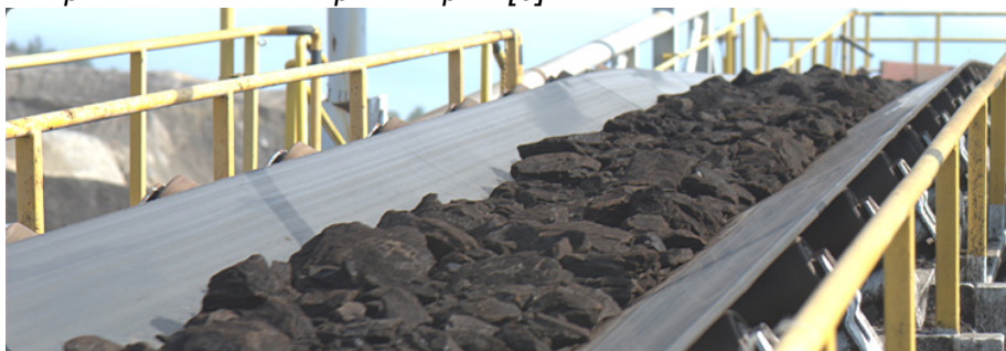
Figure 1. Conveyor belt with rubber-textile transport line
