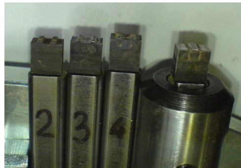
Figure 8. Fixation - shapes of deformation surfaces of tool
