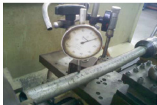
Figure 6: Measuring the deflections of the pipe by a dial gauge
