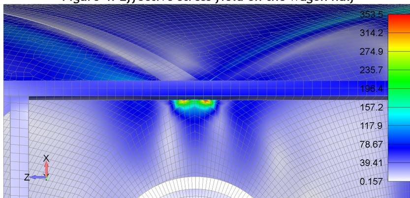
Figure 5. Effective stress field on the welding of the first tank and longitudinal girder
