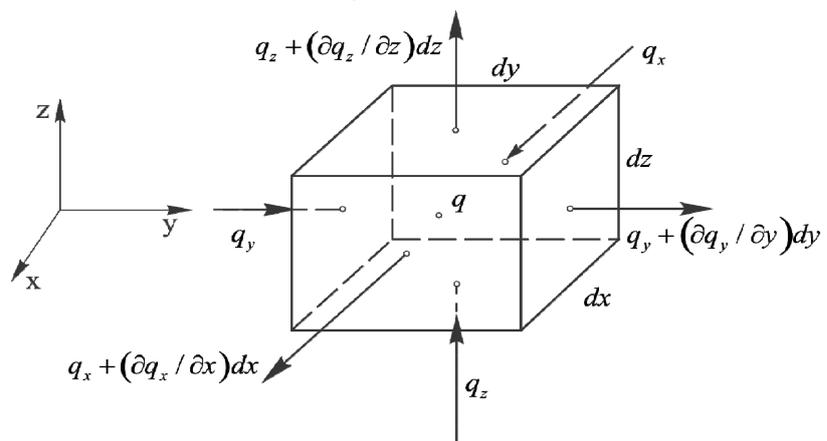
Figure 1. Elementary volume  $dV$  with heat flux components
