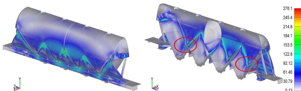
Figure 7. Effective stress field on the reconstructed model
