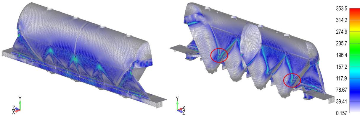
Figure 4. Effective stress field on the wagon half
