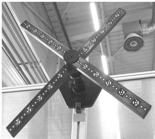
Figure 3 – Calibration cross for optical 3D scanner
