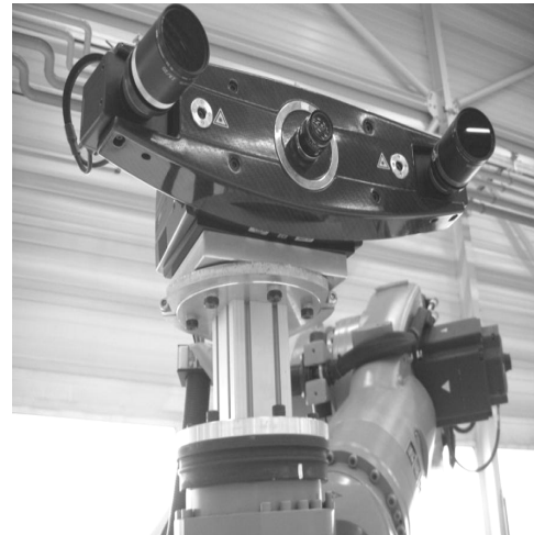
Figure 2 – Mounting adapter for optical 3D scanner on a robot arm
