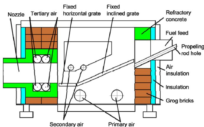
Figure 0.2 Scheme of the gasifying chamber
