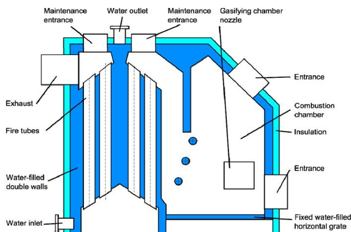
Figure 0.1. Scheme of water heater
