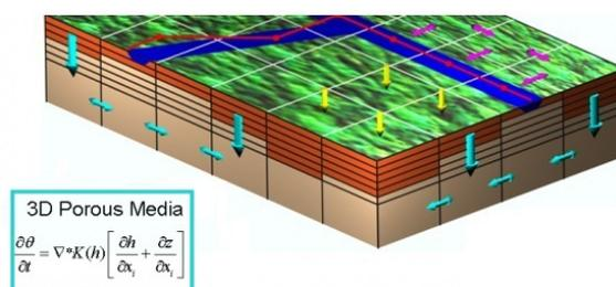
Figure 1. 3D Computer simulation for flow of water in porous media
