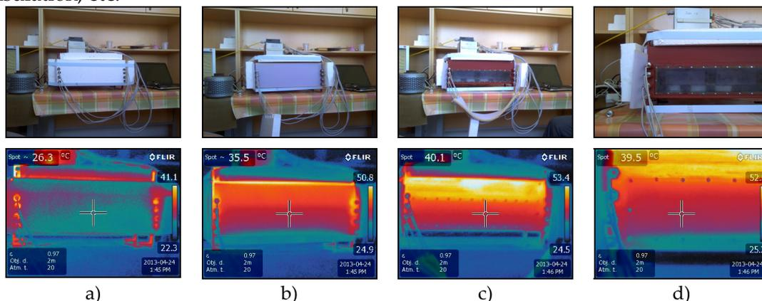
Figure 6. Temperature distribution measured with IR camera with or without insulation
