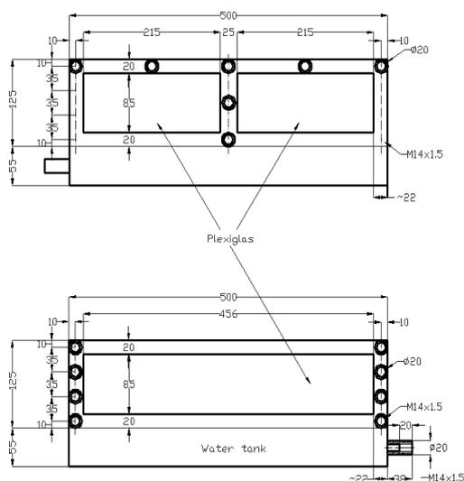
Figure 2. Disposition of the measuring points on the lateral sides of the tank
