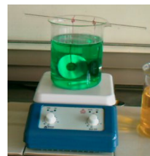
Fig. 3. Equipment for the electroless deposition of Ni composite coatings
