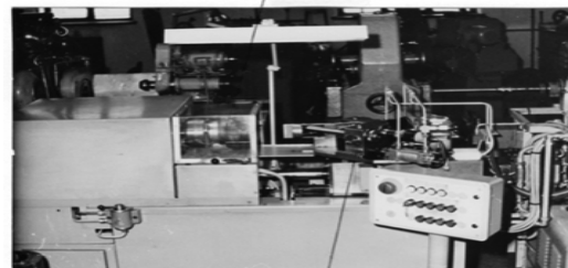
Fig. 6. The brass-coating device applied in automatic machine
