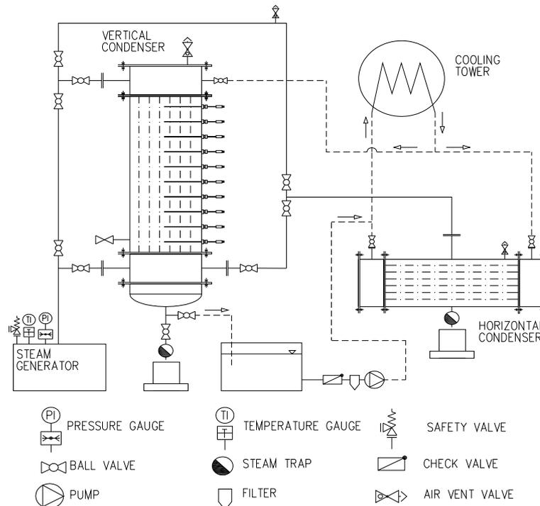
Figure 2. The general drawing of an experimental facility
