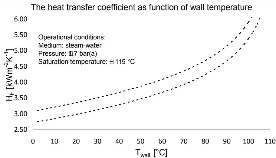
Figure 4. Expected heat transfer coefficient between two dashed lines for experiments
