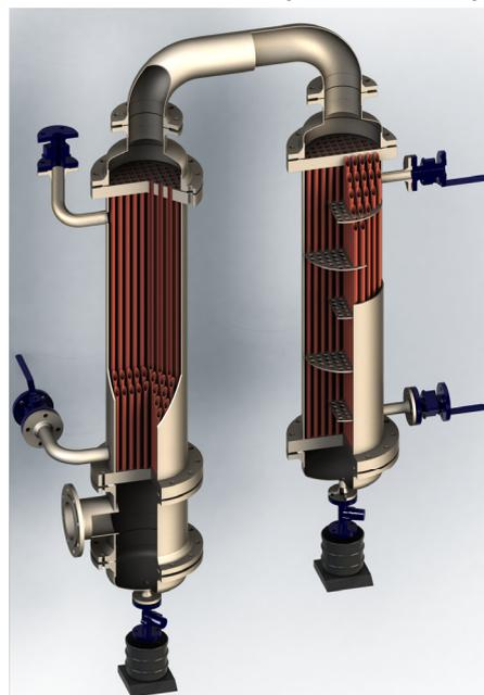
Figure 1. The experimental condenser: the left part of the heat exchanger is filled by tested PCM, the right part of the installation is cooled by water
