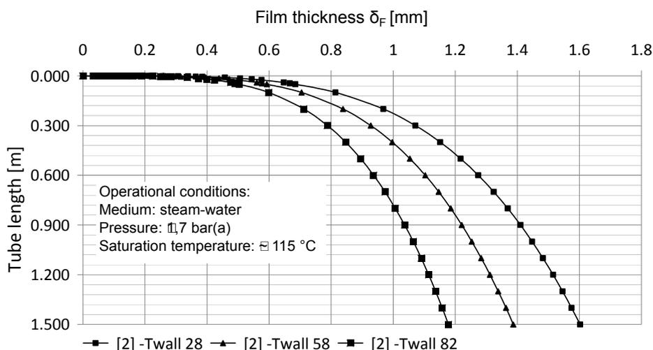
Figure 3. Expected film thickness based on the PCM material melting temperature –  $T_{wall}$
