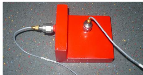
Figure 3. The mounting accelerometer to measure the acceleration in the carbody.
