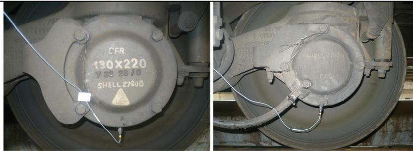
Figure 4. Mounting the accelerometers on the axle boxes
