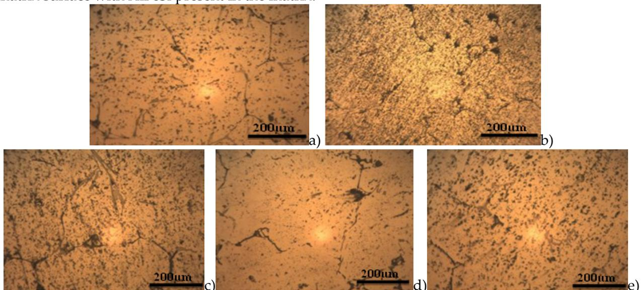
Plate 3: Microstructures of homogenized Al5Wt%Zn
