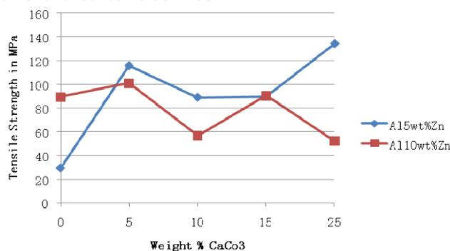
Figure 1: Ultimate tensile strength of zinc modified aluminum-0.5%Si /  $\text{CaCO}_3$  composite in as-cast state
