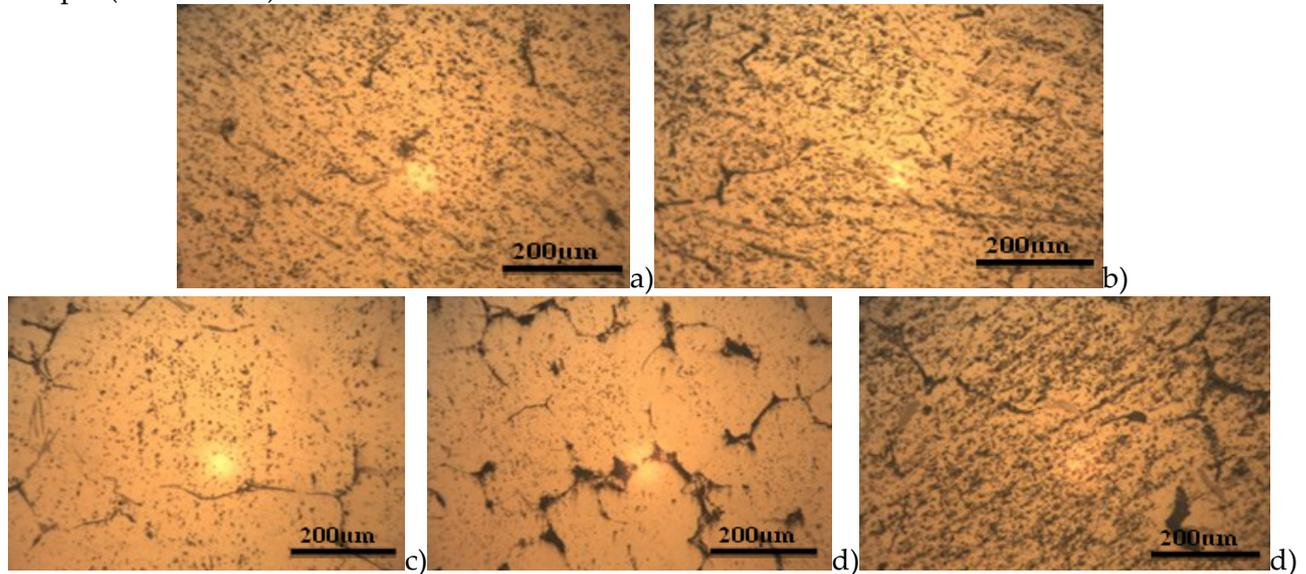
Plate 2: Microstructures of as cast Al10Wt%Zn
