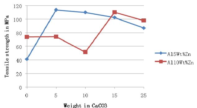
Figure 2: Ultimate tensile strength zinc modified homogenized aluminum-0.5%Si /  $\text{CaCO}_3$  composite
