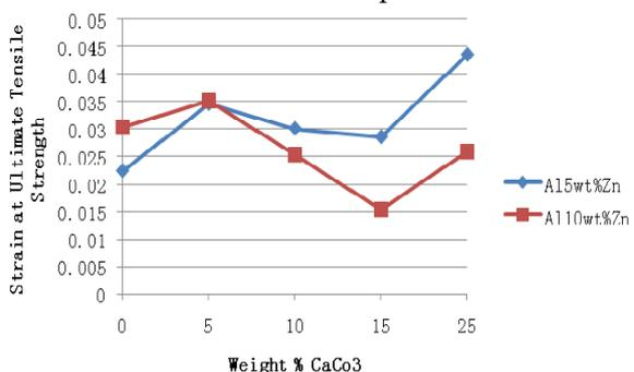
Figure 3: Strain Responses at UTS for zinc modified aluminum-0.5%Si /  $\text{CaCO}_3$  composite in as-cast state
