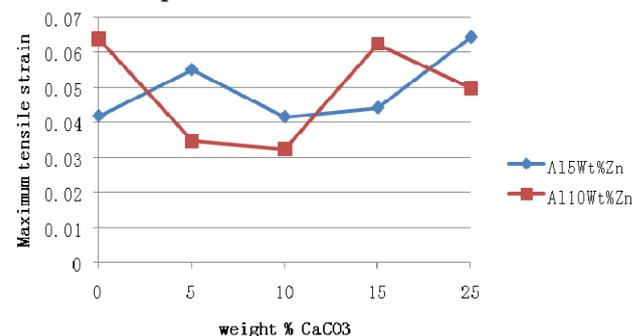
Figure 6: Maximum tensile strains for zinc modified homogenized aluminum-0.5%Si /  $\text{CaCO}_3$  composite
