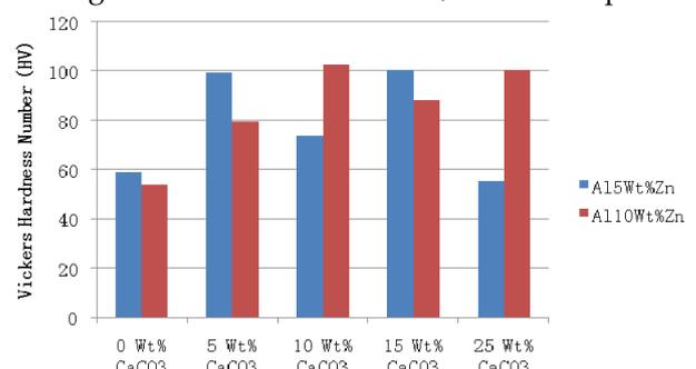
Figure 8: Hardness results (HV) of zinc modified homogenized aluminum-0.5%Si /  $\text{CaCO}_3$  composite
