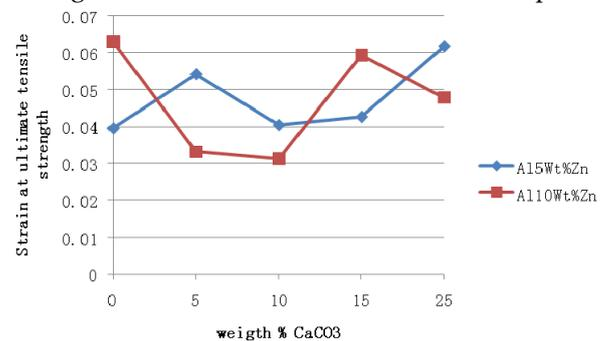
Figure 4: Strain Responses at UTS for zinc modified homogenized aluminum-0.5%Si /  $\text{CaCO}_3$  composite
