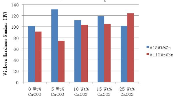
Figure 7: Hardness results (HV) of zinc modified aluminum-0.5%Si /  $\text{CaCO}_3$  composite in as-cast state
