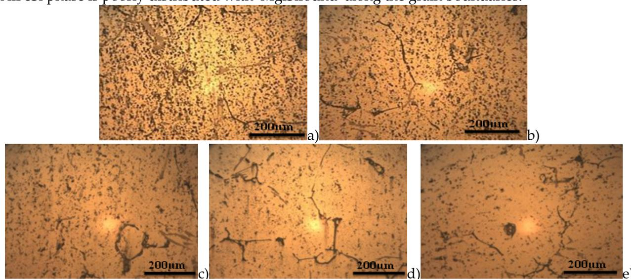
Plate 4: Microstructure of homogenized Al10Wt%Zn
