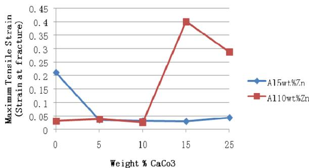
Figure 5: Maximum tensile strains for zinc modified aluminum-0.5%Si /  $\text{CaCO}_3$  composite in as-cast state
