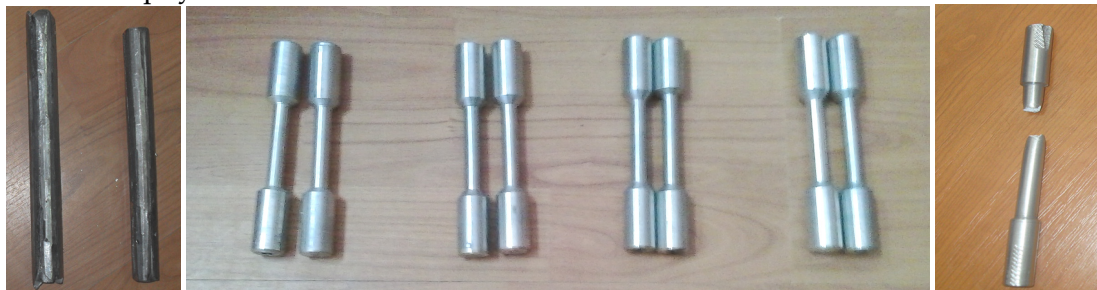
Figure 6. Forging and machining the samples
