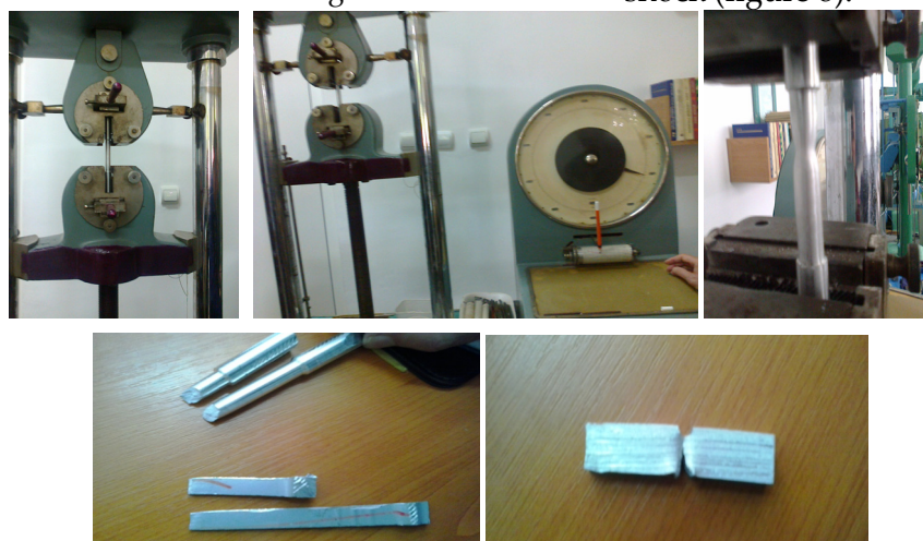
Figure 8. Specimens used for tensile testing and impact bend
