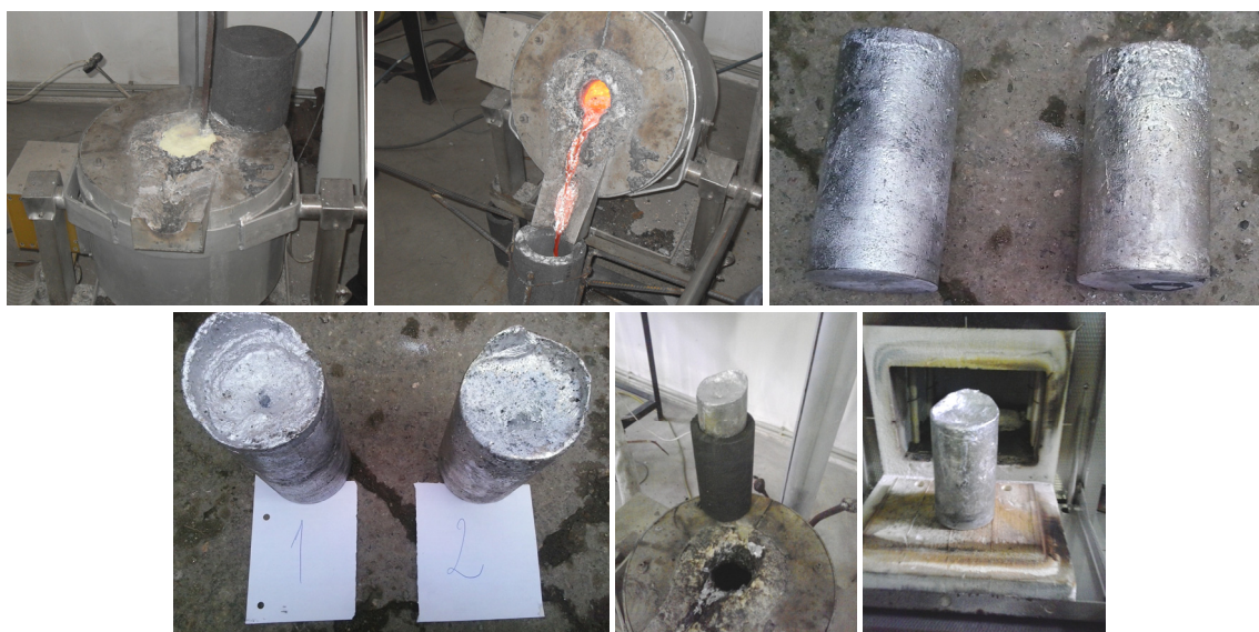
Figure 5. Aspects of drafting and casting aluminum alloy
