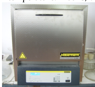
a) melting furnace (calcination) Nabertherm model L15/12/B180;
