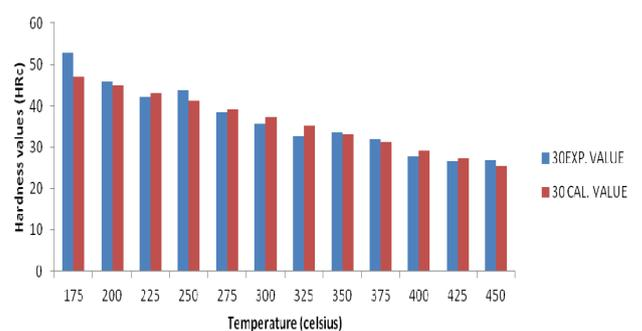
Fig. 2 : Variation of Hardness Values with Temperature for both Experimental (Exp.) and Calculated (CAL.) values
