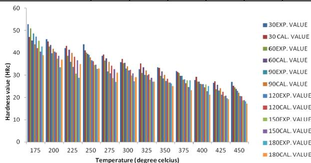
Fig. 1: Variation of Hardness Values with Immersion Temperature of Ductile Iron
