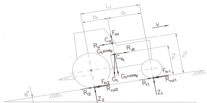
Fig. 1 - Tractor running on a sloped field which suddenly brakes
