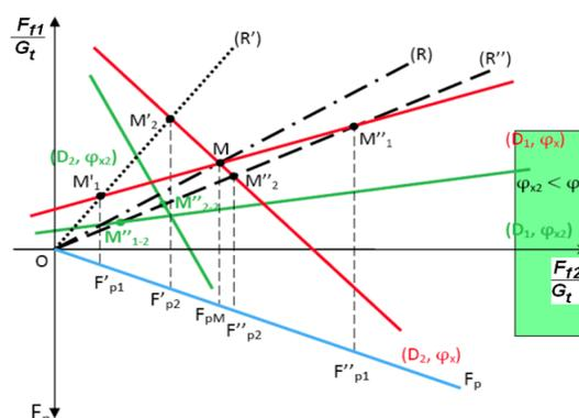
Fig. 3 – Equation of straight line repartition at shaft axles [1]
