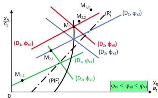
Fig. 4 – Equation of braking parabola [1]
