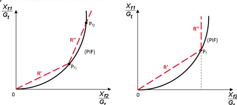
Fig. 5 - Approximation (PIF) of pressure transmitted to braking mechanisms of rear shaft wheels
