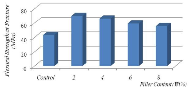
Figure 3: Variation of flexural strength at fracture with filler content for the varied steelmaking slag particles
