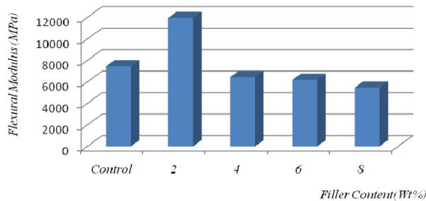
Figure 2: Variation of flexural modulus with filler content for the varied steel making slag particles
