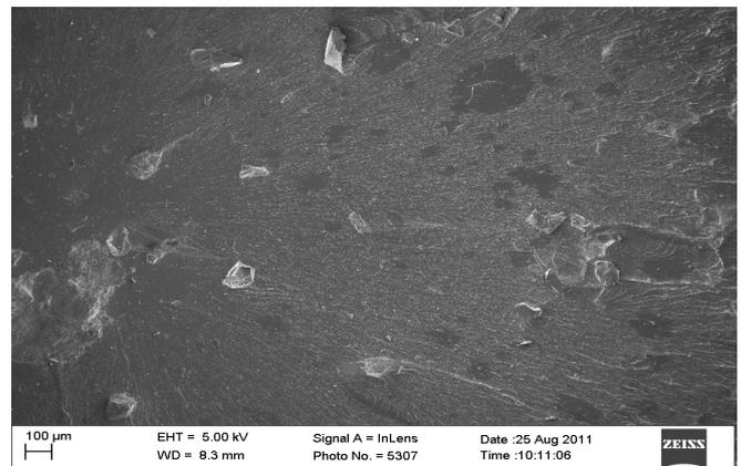
Figure 4: SEM micrograph of fractured surface of 2 wt% steelmaking slag filled polyester Composites
