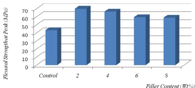
Figure 1: Variation of flexural strength at peak with filler content for the varied steel making slag particles
