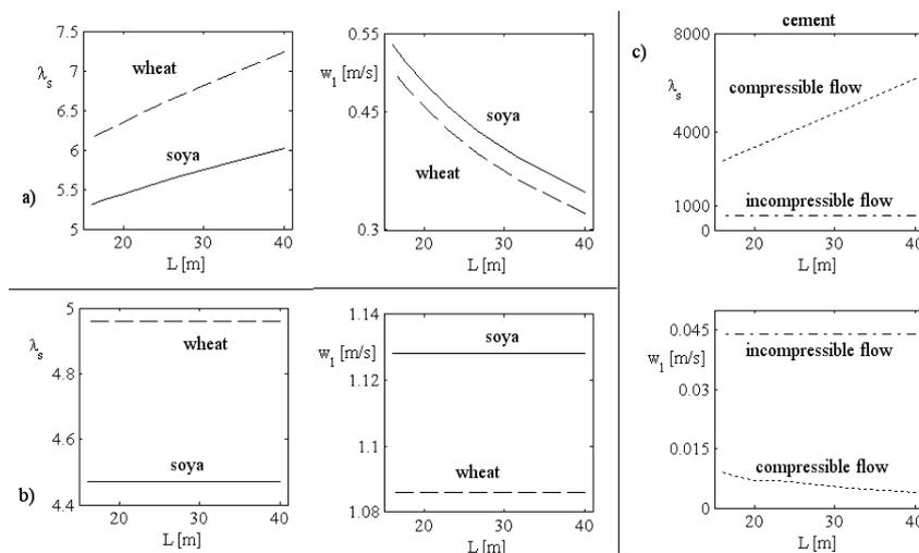
Figure 2. The effect of the calculation method on the air velocity and friction coefficient: a) compressible flow, b) incompressible flow, c) cement
