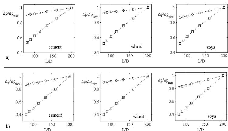
Figure 3. Sensitivity of pressure drop on the change of air-lift's pipe diameter and lifting height of the material: a) calculation based on the compressible air flow, b) calculation based on the incompressible air flow; circle- change in diameter, square- change of height
