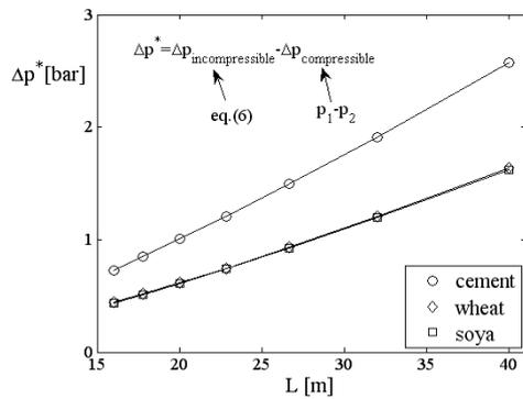
Figure 1. The difference in calculated pressure drop depending on the calculation method
