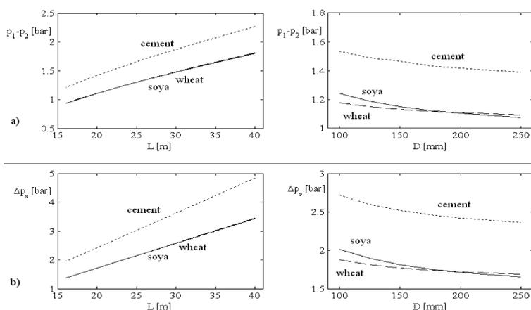
Figure 4. The influence of air-lift's diameter and lifting height on the values of pressure drop: a) compressible flow of air, b) incompressible air flow
