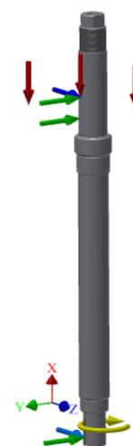
Figure 3. Loading of the spindle
