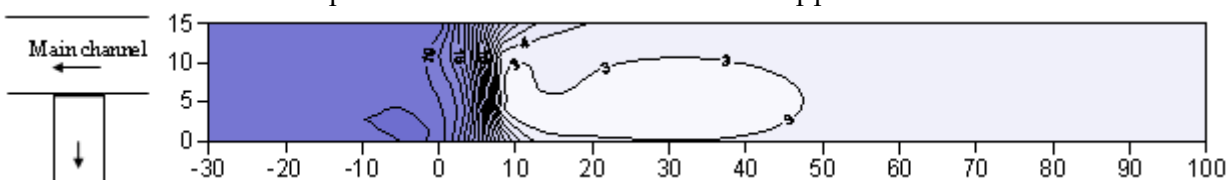
Fig. (25) water surface elevation for normal side weir of P=12 cm
