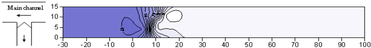
Fig. (39) water surface elevation for triangular side weir of P=12\text{cm} & \theta=75^\circ opposite direction of flow
