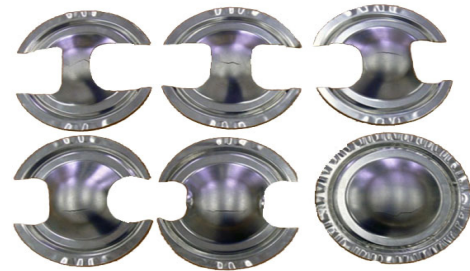
Fig. 8. Dog bone shaped specimens for Nakajima test to determine FLC curve
