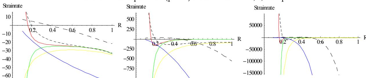
Figure 14. Thermal creep strain rates ( $\theta_1 = 3$ ) for a non-homogeneous thick-walled circular cylinder under external pressure ( $p = 50$ ) for measure  $N = 1, 2, 5$  resp.
