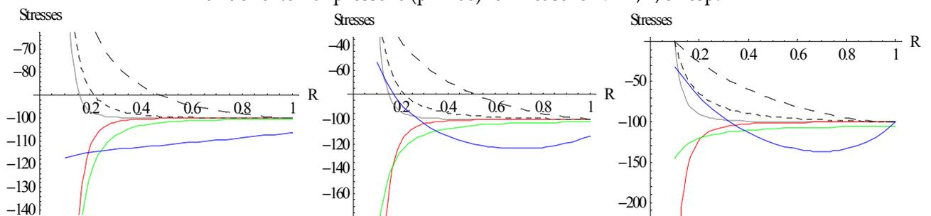
Figure 4. Creep Stresses without temperature for a non-homogeneous thick-walled circular cylinder under external pressure ( $p = 100$ ) for measure  $N = 1, 2, 5$  resp.
