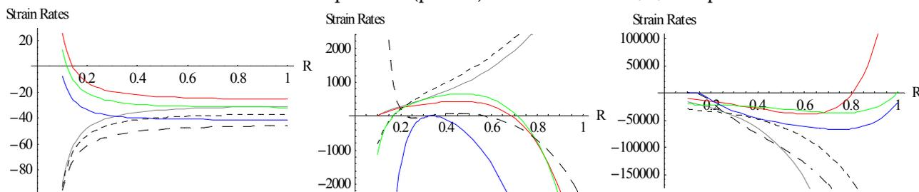
Figure 13. Thermal creep strain rates ( $\theta_1 = 3$ ) for a homogeneous thick-walled circular cylinder under external pressure ( $p = 50$ ) for measure  $N = 1, 2, 5$  resp.
