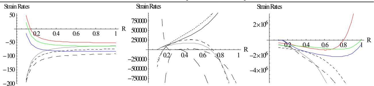
Figure 15. Thermal creep strain rates ( $\theta_1 = 3$ ) for a homogeneous thick-walled circular cylinder under external pressure ( $p = 100$ ) for measure  $N = 1, 2, 5$  resp.
