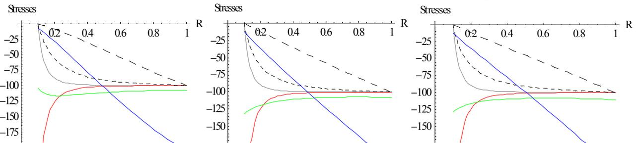
Figure 8. Thermal creep Stresses ( $\theta_1 = 3$ ) for a non-homogeneous thick-walled circular cylinder under external pressure ( $p = 100$ ) for measure  $N = 1, 2, 5$  resp.
