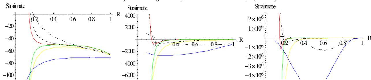
Figure 12. Creep strain rates without temperature for a non-homogeneous thick-walled circular cylinder under external pressure ( $p = 100$ ) for measure  $N = 1, 2, 5$  resp.
