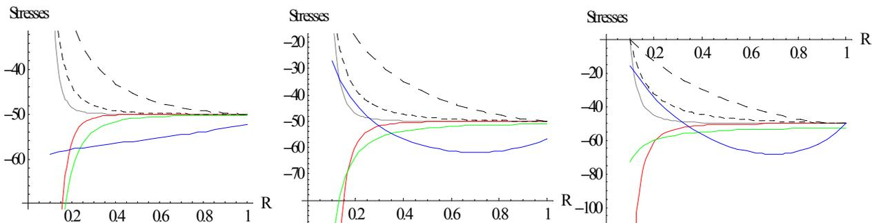
Figure 2. Creep Stresses without temperature for a non-homogeneous thick-walled circular cylinder under external pressure (p = 50) for measure N = 1, 2, 5 resp.
