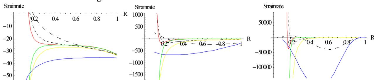
Figure 10. Creep strain rates without temperature for a non-homogeneous thick-walled circular cylinder under external pressure ( $p = 50$ ) for measure  $N = 1, 2, 5$  resp.
