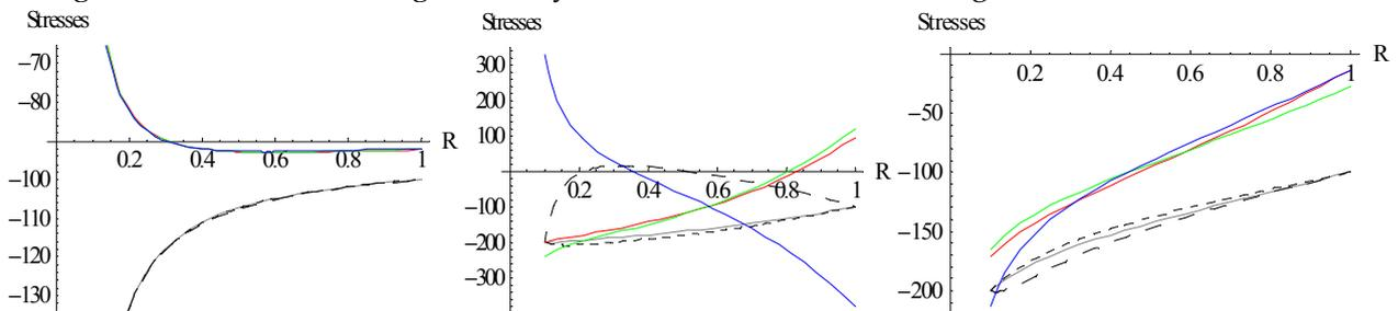
Figure 7. Thermal creep Stresses ( $\theta_1 = 3$ ) for a homogeneous thick-walled circular cylinder under external pressure ( $p = 100$ ) for measure  $N = 1, 2, 5$  resp.
