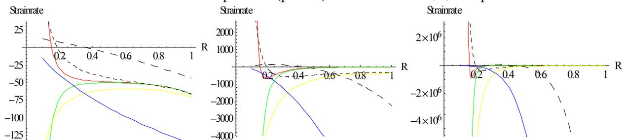
Figure 16. Thermal creep strain rates ( $\theta_1 = 3$ ) for a non-homogeneous thick-walled circular cylinder under external pressure ( $p = 100$ ) for measure  $N = 1, 2, 5$  resp.
