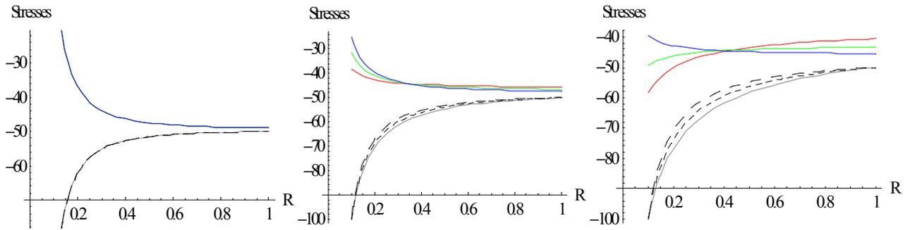
Figure 1. Creep Stresses without temperature for a homogeneous thick-walled circular cylinder under external pressure (p = 50) for measure N = 1, 2, 5 resp.
