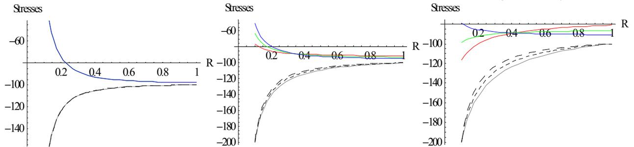
Figure 3. Creep Stresses without temperature for a homogeneous thick-walled circular cylinder under external pressure ( $p = 100$ ) for measure  $N = 1, 2, 5$  resp.
