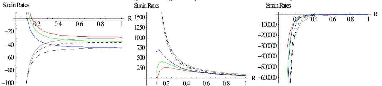
Figure 9. Creep strain rates without temperature for a homogeneous thick-walled circular cylinder under external pressure ( $p = 50$ ) for measure  $N = 1, 2, 5$  resp.
