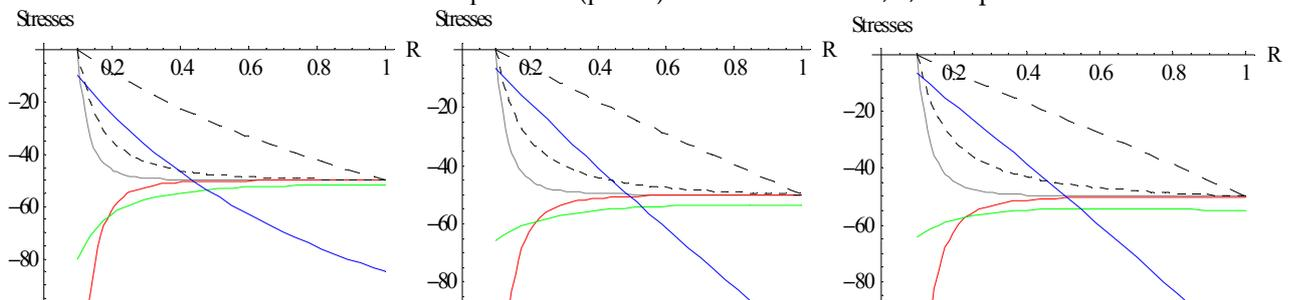
Figure 6. Thermal creep Stresses ( $\theta_1 = 3$ ) for a non-homogeneous thick-walled circular cylinder under external pressure ( $p = 50$ ) for measure  $N = 1, 2, 5$  resp.
