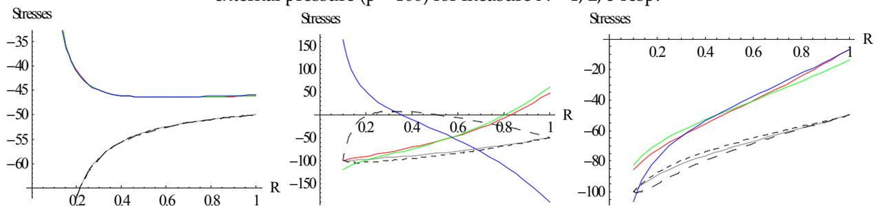
Figure 5. Thermal creep Stresses ( $\theta_1 = 3$ ) for a homogeneous thick-walled circular cylinder under external pressure ( $p = 50$ ) for measure  $N = 1, 2, 5$  resp.
