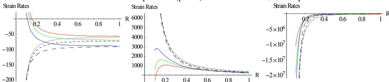
Figure 11. Creep strain rates without temperature for a homogeneous thick-walled circular cylinder under external pressure ( $p = 100$ ) for measure  $N = 1, 2, 5$  resp.
