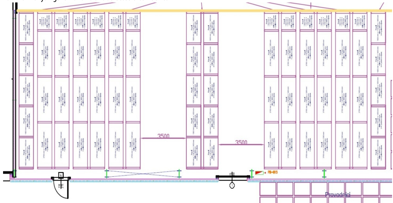
Figure 4 – The variant with 2 block movable racks and reach truck
