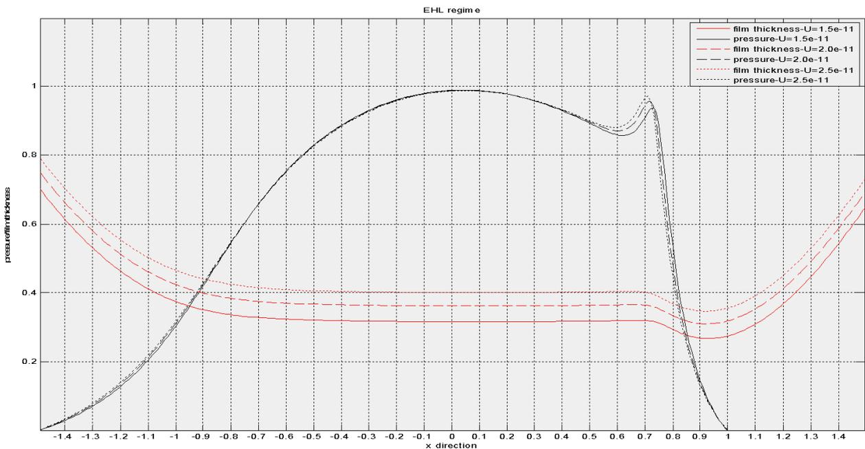
**Figure 3:** Film thickness profile and pressure distribution comparison using Roelands' law, with  $U=1.5 \times 10^{-11}$  (solid line);  $U=2.0 \times 10^{-11}$  (dashed line),  $U=2.5 \times 10^{-11}$  (dot line)
