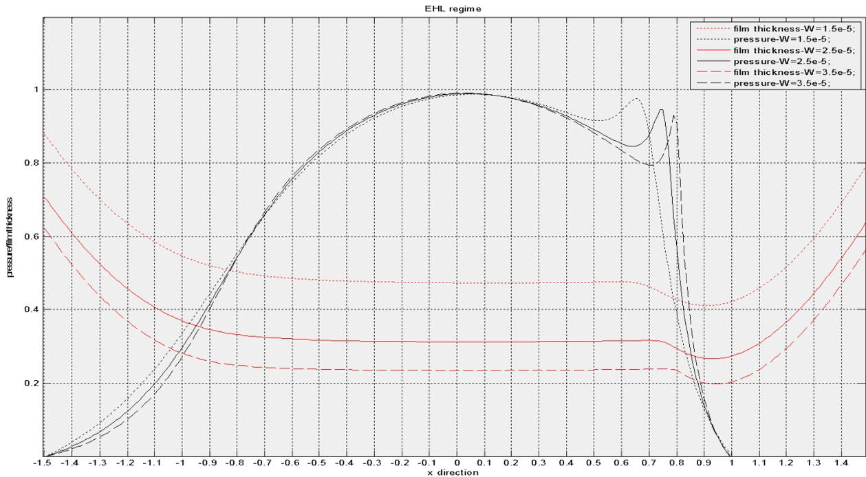
**Figure 2:** Film thickness profile and pressure distribution comparison using Roelands' law, with  $W=1.5 \times 10^{-4}$  (dot line);  $W=2.5 \times 10^{-4}$  (solid line),  $W=3.5 \times 10^{-4}$  (dashed line)
