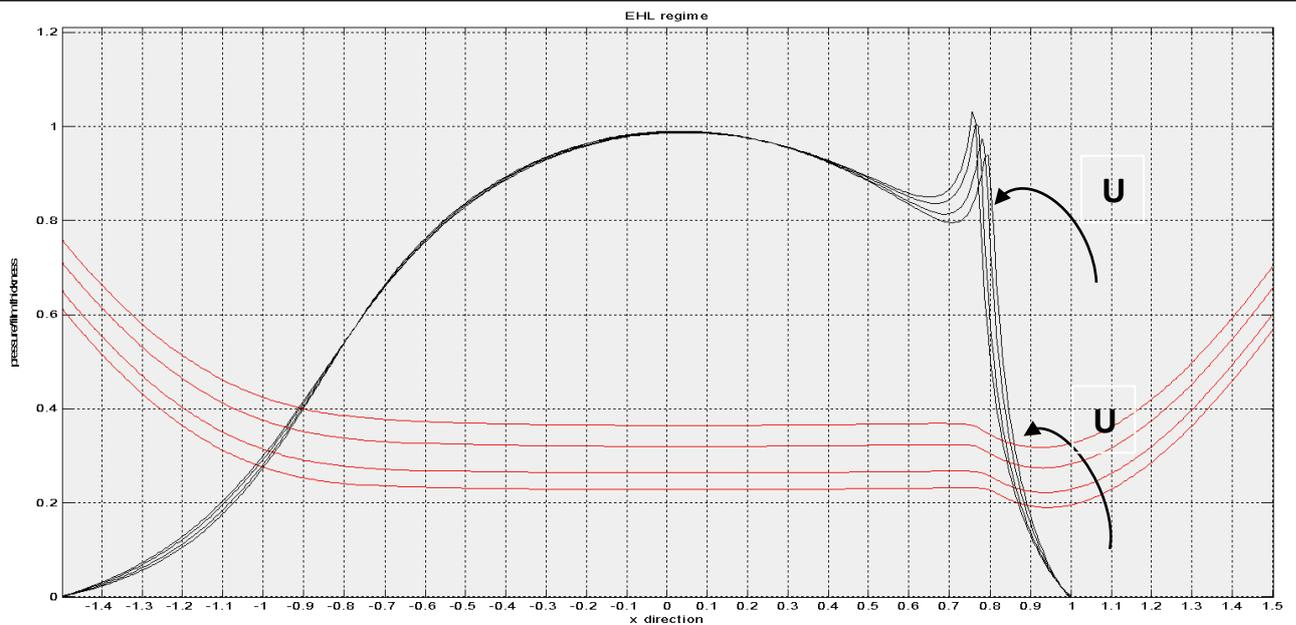
**Figure 5:** Film thickness profile (red line) and pressure distribution (black line) comparison using Doolittle model for different level of dimensionless sliding speed (from  $U=1.0 \times 10^{-11}$  to  $U=6.0 \times 10^{-11}$ )
