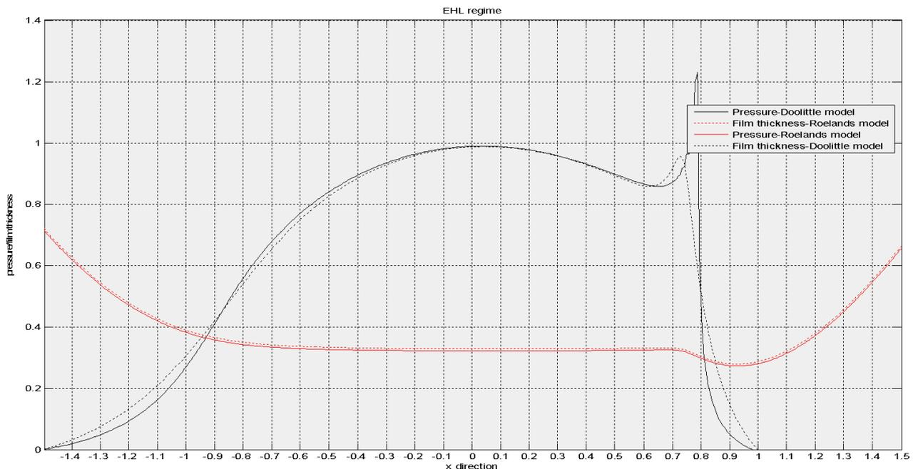
**Figure 6:** Film thickness profile and pressure distribution using Doolittle' model (solid line) and Reolands' law (dashed line) with  $W=3.0 \times 10^{-4}$ ;  $U=2.0 \times 10^{-11}$ .
