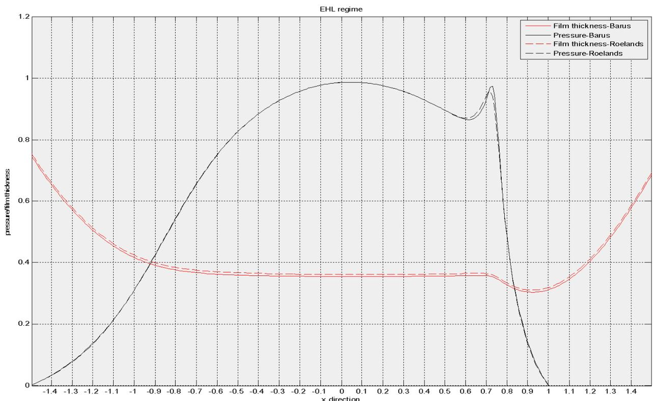
Figure 1: Film thickness profile and pressure distribution using Roelands' law (solid line) and Barus law (dashed line) with  $W=3.0 \times 10^{-4}$ ;  $U=2.0 \times 10^{-11}$ .
