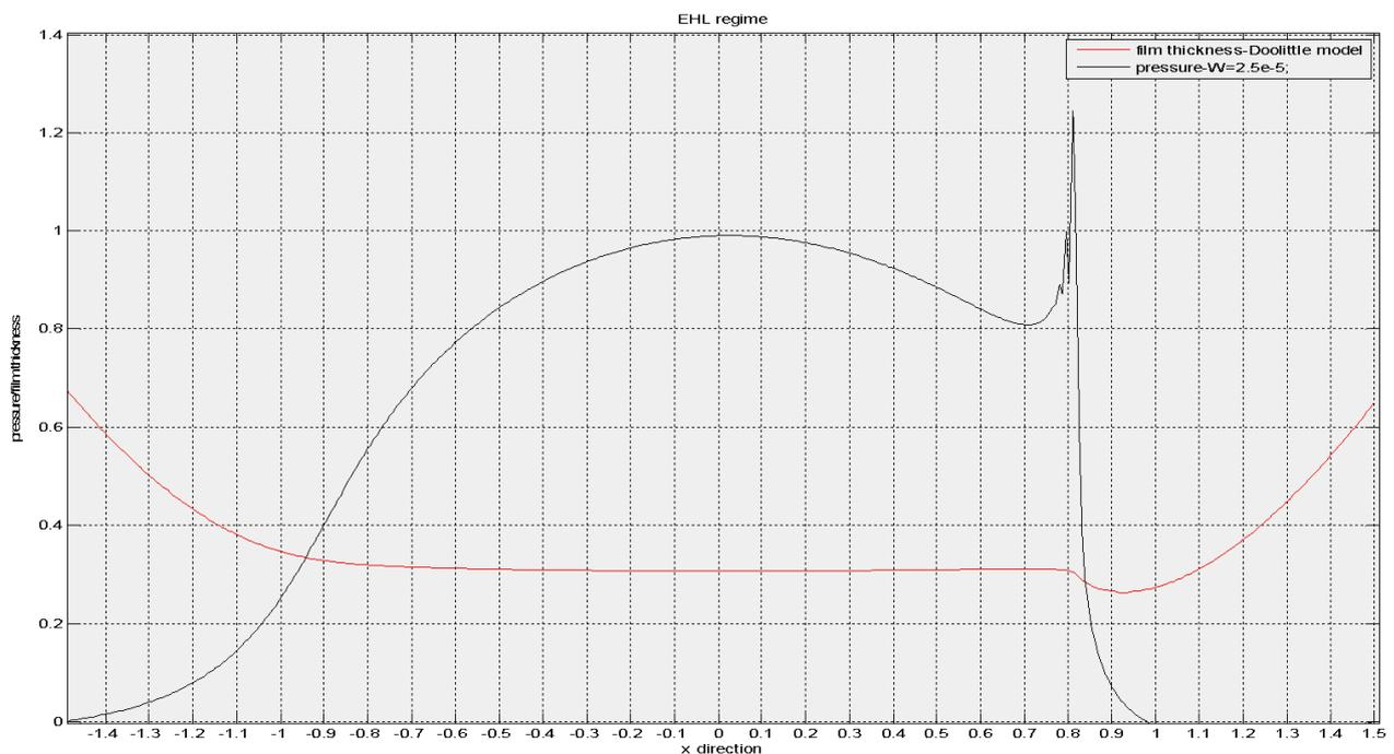
**Figure 4:** Film thickness profile and pressure distribution using Doolittle model with  $W = 3.0 \times 10^{-4}$ ;  $U = 2.0 \times 10^{-11}$ .
