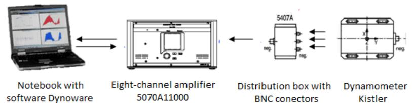
**Figure 8:** The Kistler data acquisition and processing [6]
