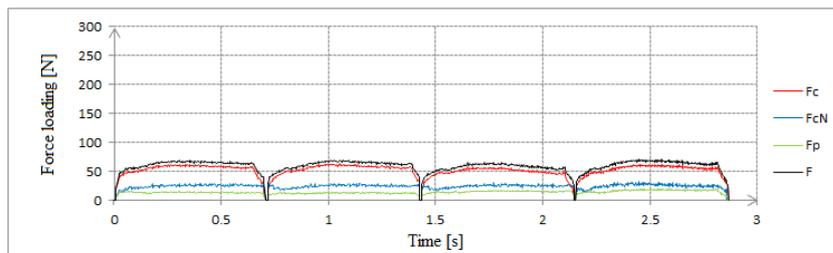
**Figure 11:** Time series of the force loading for the milling cutter (producer ZPS-FN, Zlín, CZ); machining of artificial wood SikaBlock M610.
