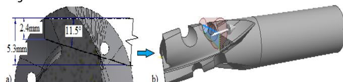
Figure 5: Used cone for rotation and finished compensation edges
