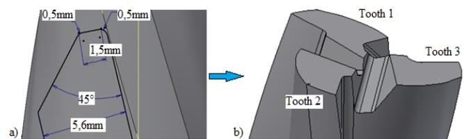
Figure 3: Sketch of used grinding wheel and finished face surfaces
