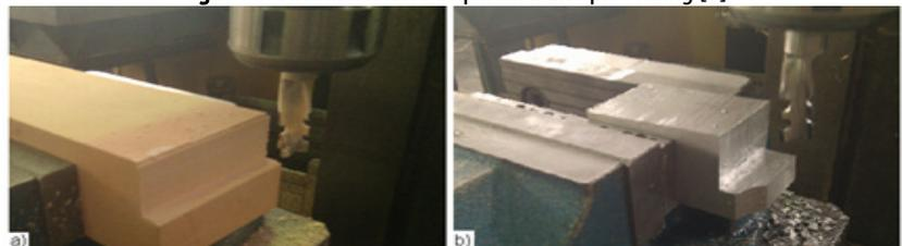
**Figure 9:** Workpiece and tool clamping
