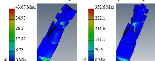
**Figure 14:** Stress analysis: a) for data measured during machining of artificial wood; b) for data measured during machining of aluminium alloy.
