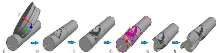
Figure 2: Construction of helical groove
