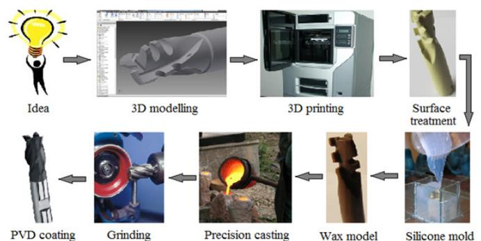
Figure 1: Designed technology of production of new cutting tool with compensation edges
