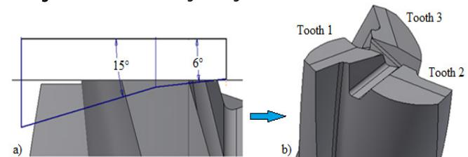
Figure 4: Sketch used for extruding and finished flank surfaces
