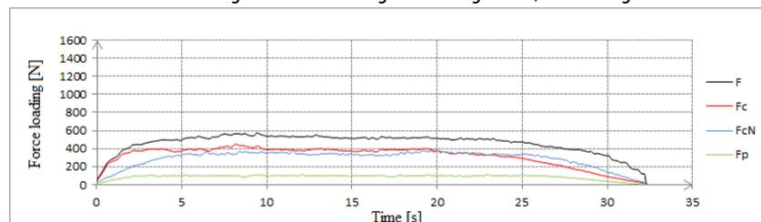
**Figure 13:** Time series of the force loading for the milling cutter (producer ZPS-FN, Zlín, CZ); machining of aluminium alloy AlCu4MgSi.
