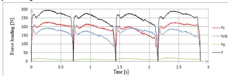
**Figure 10:** Time series of the force loading for the new designed milling cutter; machining of artificial wood SikaBlock M610.
