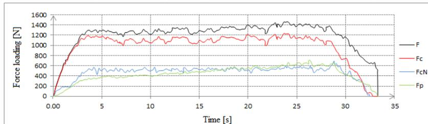
**Figure 12:** Time series of the force loading for the new designed milling cutter; machining of aluminium alloy AlCu4MgSi.
