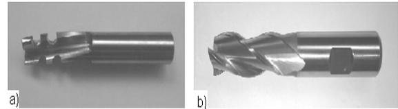
**Figure 7:** Tested milling cutters: a) with compensation edges; b) tool made by ZPS-FN
