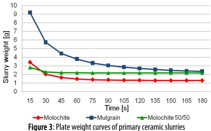
Figure 3: Plate weight curves of primary ceramic slurries
