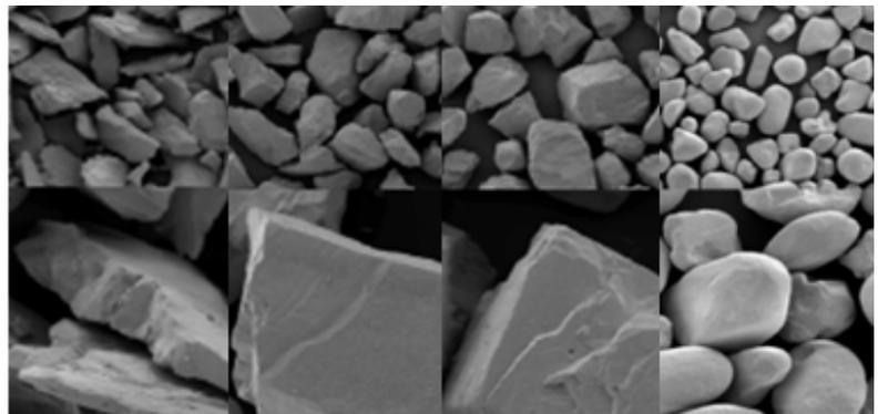
Figure 2: Particle shape analysis of refractory materials [6]
