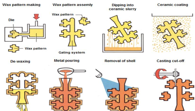
Figure 1: Principle of lost wax technology [3]
