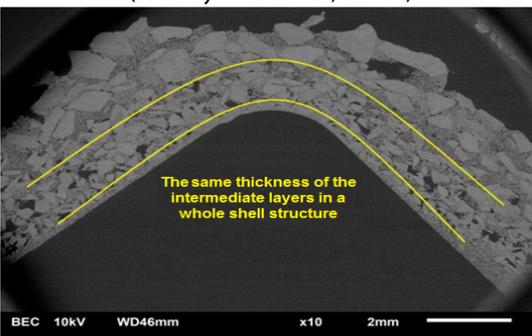
**Figure 8:** SEM picture of corner of newly developed ceramic shell
