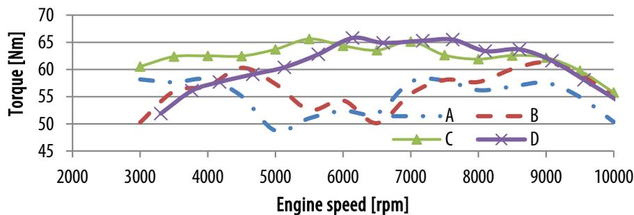
**Figure 12.** Comparison of torque characteristics of simulations and measurement
