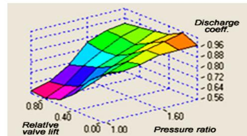
Figure 3. Extrapolated map of Discharge Coefficient as a function of relative valve lift and pressure ratio across the valve
