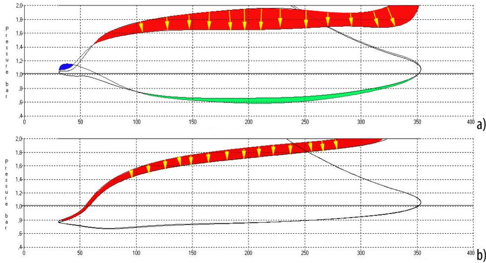
**Figure 8. a-b.** P-V diagrams of the gas exchange process showing the decrease in pumping losses in red. The green area represents a small improvement in the strength of the intake stroke realized by the smaller amount of exhaust gas back flow.
