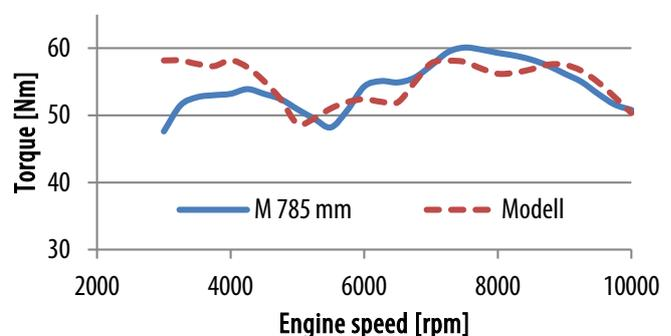
Figure 5. Comparison of measured and simulated torque curves obtained using the 785 mm exhaust pipe
