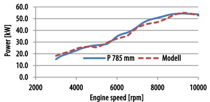
Figure 4. Comparison of measured and simulated power curves obtained using the 785 mm exhaust pipe
