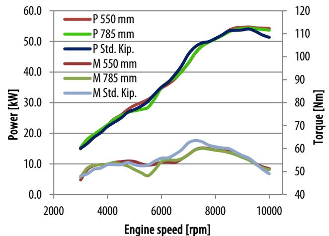
**Figure 1.** Power and torque characteristics of the engine with the OEM and the two manufactured exhaust systems
