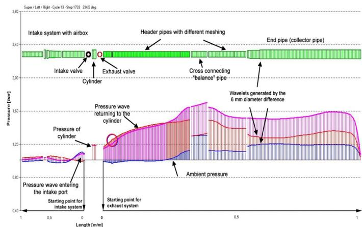
**Figure 7.** Animation showing cylinder #1 at when the exhaust pressure wave enters the intake port causing back flow and diluting fresh charge with exhaust gas. The red circle shows wavelets produced by a welding protruding into the exhaust flow. Purple shows the superonated pressure, blue the returning (leftward) waves, red is the escaping (rightward) pressure waves
