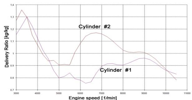
Figure 6. Delivery ratio curves for both cylinders
