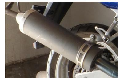
**Figure 10.** Silencer manufactured based on the results of simulation
