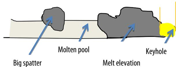
**Figure 8:** Video and scheme of melt elevation for SCM420– WS3 weld
