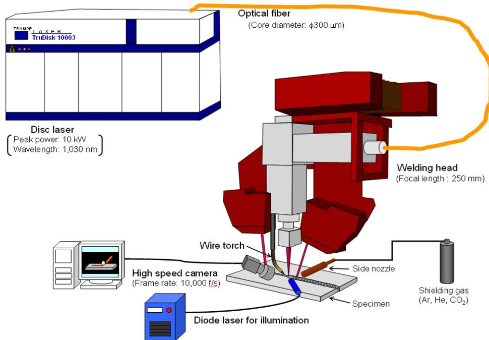
Figure 2: Welding setup – TruDisk 10003 and HighYAG welding head
