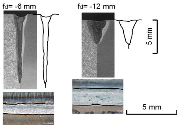
Figure 11: V shaped cross sections and bead views of samples with focal point deeply in material
