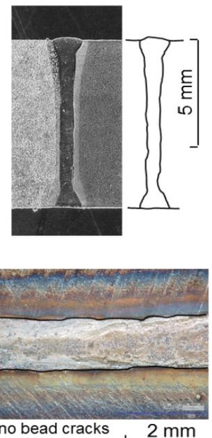
Figure 12: Full penetration weld – sample thick 8 mm, cross sections, upper view of the bead surface
