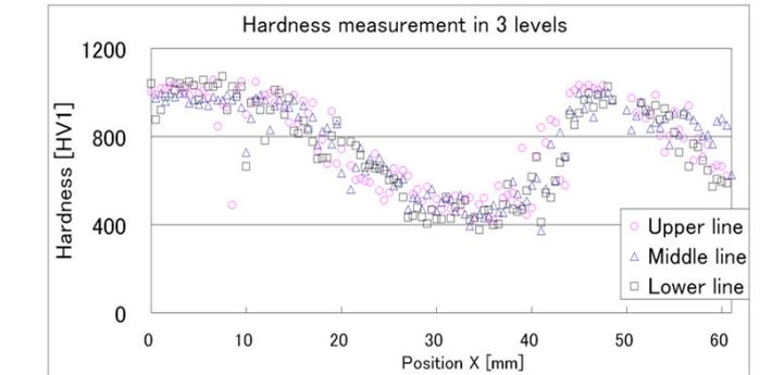
Figure 10: Evolution of hardness along misaligned weld (longitudinal section)
