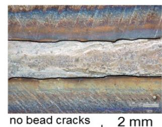
Figure 12: Full penetration weld – sample thick 8 mm, cross sections, upper view of the bead surface
