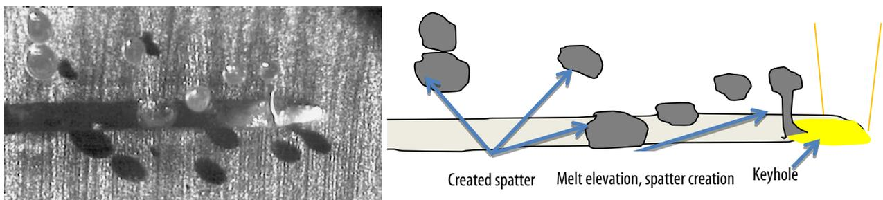
Figure 5: Video and scheme of melt elevation as taken by high speed camera
