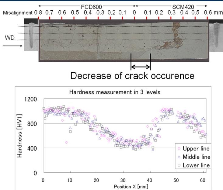
Figure 10: Evolution of hardness along misaligned weld (longitudinal section)
