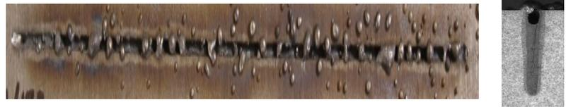
Figure 4: Weld 8 kW, 50 mm/s, fd=0 mm, high formation of spatter and underfill
