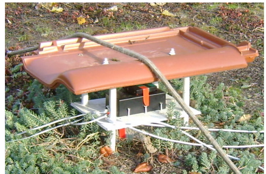
Figure 3 - Electronical unit with weather protection, battery, and wires
