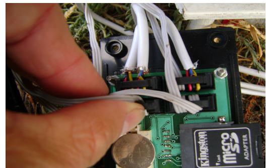
Figure 4 - PIC18F4550 type micro controller unit with wires, SD memory card and CR2032 battery for the clock
