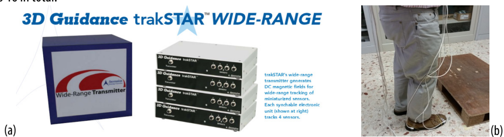
Figure 7. trakSTAR WIDE-RANGE measuring equipment with DC magnetic field transmitter [11] (a); remote sensor during measuring experiment (b)
