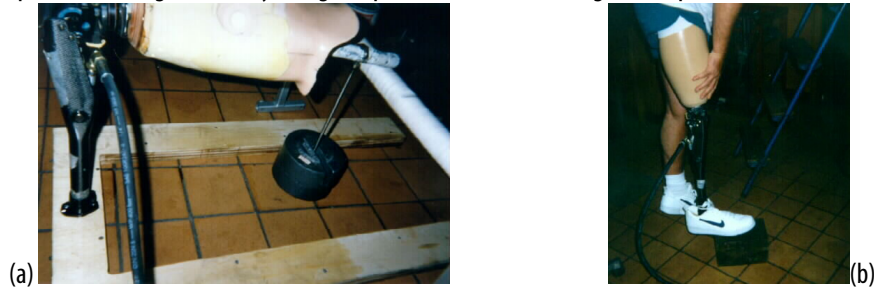
Figure 1. Experimental testing of prosthesis with hydraulic actuator integrated in the knee: in laboratory conditions (a) and in real operating conditions (b) [2,3]
