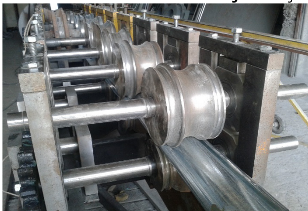
Figure 8. Picture of reconstructed machine for the production of specialized profile
