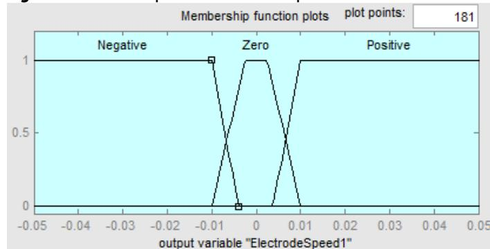
**Figure 5.** Membership functions for the output variable *Electrode Speed*
