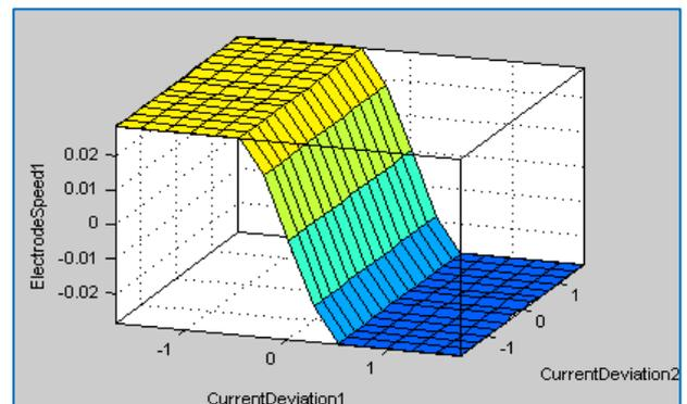
Figure 8. The surface obtained with the fuzzy system for two inputs and one output
