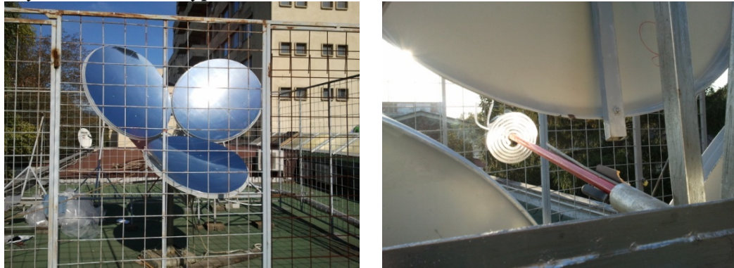
Figure 5. a) Experimental model of a parabolic offset solar concentrator system; b) The concentration of solar radiation in a spiral absorber
