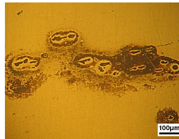
a) Sample 1.2.3 (without etching), longitudinal section, coarse non-metallic inclusions of A3, B1 and D2 type.
