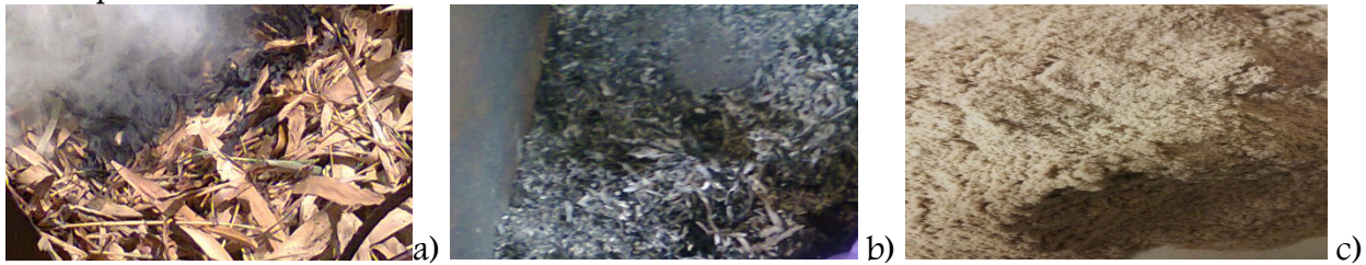
Figure 1. a) burning dried bamboo leaf. b) as-received bamboo leaf ash. c) bamboo leaf ash after conditioning in muffle furnace at a temperature of 650 °C for 3 hours.
