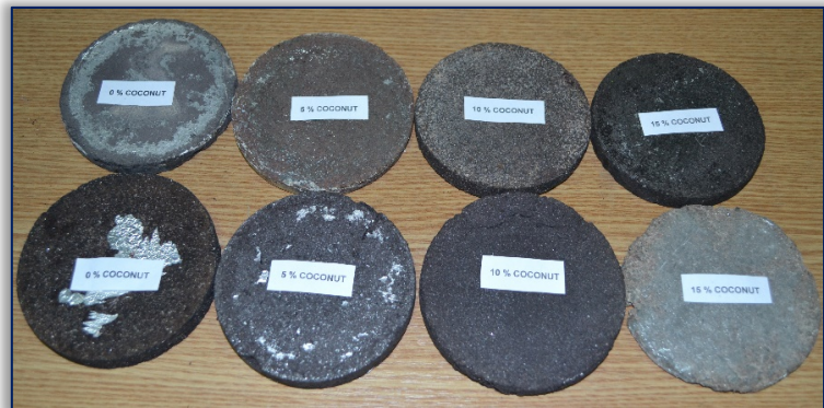
Figure 4. The presentation of two sets of samples with variable addition of coconut fiber
