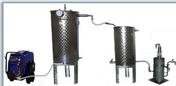
Figure 1 – Distillation plant with pressurized steam generator
