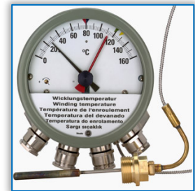
Figure 8. Winding temperature indicator (WTI)
