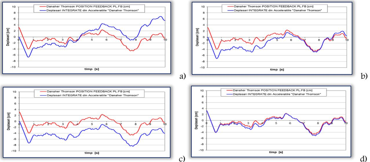
Figure 2: Repeated attempts for identifying the two integration constants to obtain a correct displacement by double integration of acceleration: a)  $C_x(t_0)=0$ ,  $C_v(t_0)=0$  (step 1); b)  $C_x(t_0)=0$ ,  $C_v(t_0)=-0.5$  (step 2); c)  $C_x(t_0)=0$ ,  $C_v(t_0)=-0.95$  (step 2); d)  $C_x(t_0)=3.3$ ,  $C_v(t_0)=-0.95$  (step 4).
