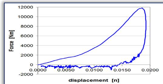
Figure 4: Force-displacement curve for the impact of a flat rubber mat with a spherical impactor head, obtained only from acceleration measurements
