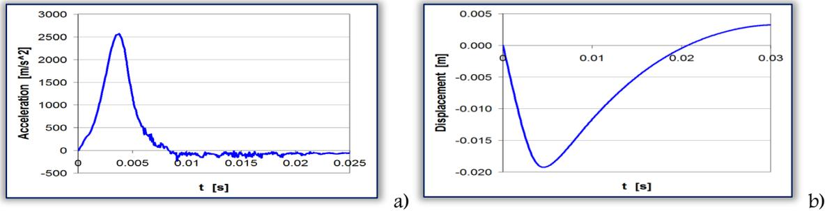
Figure 3: Impact of a flat rubber mat with a spherical impactor head: a) measured vertical acceleration; b) vertical displacement obtained by numerical double integration of the measured acceleration
