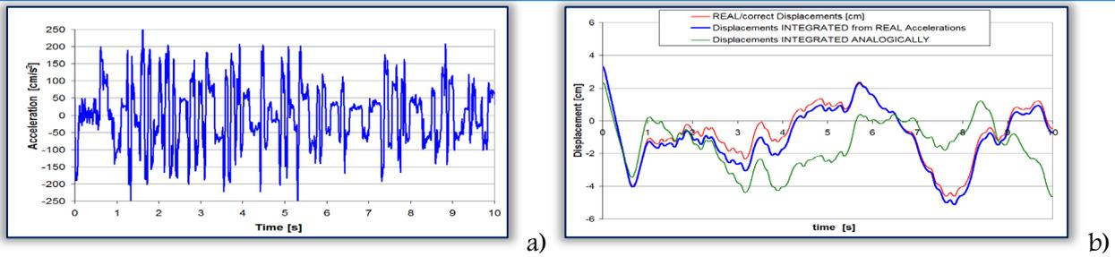
Figure 1: a) Driver seat accelerations for a car ride simulated using CARSIM [5]; b) Driver seat displacements: “real” ones, the ones integrated from the “real” accelerations and the ones integrated analogically by our data acquisition system
