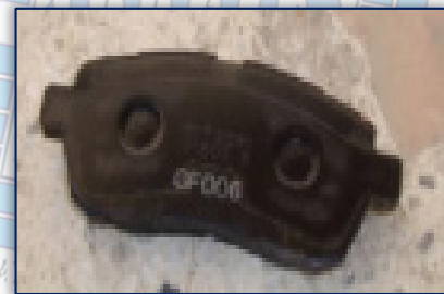
Figure 22. The brake pad made of composite material under test in the experimental installation
