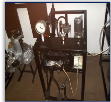
Figure 16. The general assembly of experimental installation for testing composite materials
