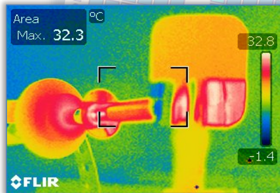
Figure 8. Comparative Thermal imager tests; a – coated intake section probe, b – no coated intake section probe
