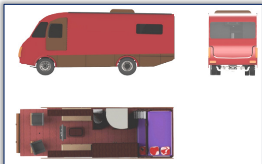
Figure 4: Orthographic view of proposed motorhome for Indian families (in first quadrant projection system)
