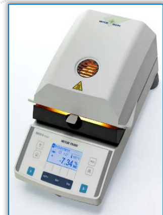
Figure 1: Halogen moisture analyser METTLER TOLEDO HB43-S
