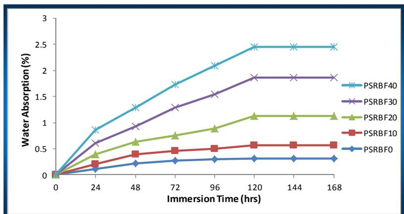
Figure 7: Water Absorption Curves for the Polyester/SRBF Composites
