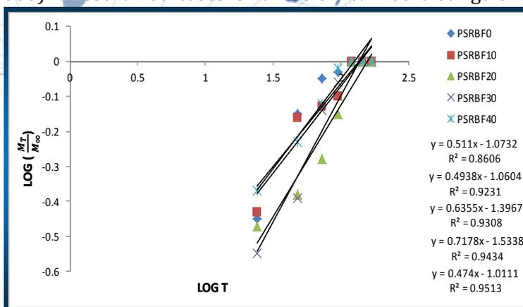
Figure 8: Diffusion Curve Fitting Plot for the Polyester/SRBF Composites
