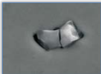
Figure 6. Nucleation of microcavities of with mechanism of decohesion and fracture [16]
