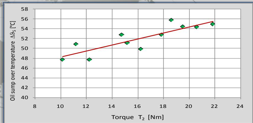
Figure 4. The change flow in the increase of oil temperature  $\Delta\vartheta_s$  obtained by means of an experiment for the rotation speed of  $n_1 = 5000 \text{ min}^{-1}$  and for different values of the output torque of  $T_2$
