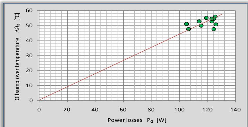
Figure 5. The change flow in the increase of oil temperature  $\Delta\vartheta_s$  obtained by means of an experiment for the rotation speed of  $n_1=5000\text{min}^{-1}$  and for different values of the output torque  $T_2$
