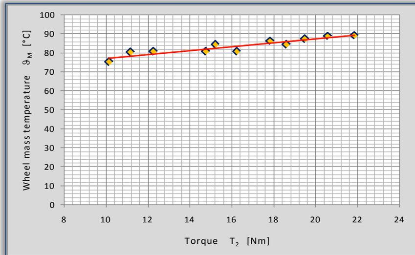
Figure 6. The change flow in the wheel mass temperature  $\vartheta_M$  for the rotation speed  $n_1=5000$   $\text{min}^{-1}$  and for different values of the output torque  $T_2$  as a result of increased power losses, the wheel mass temperature  $\vartheta_M$  increases as well.
