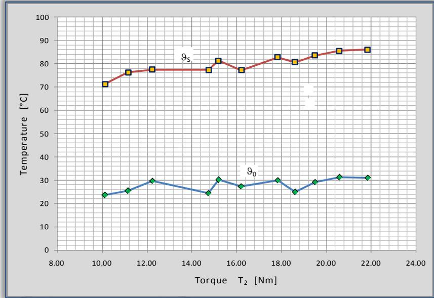
Figure 3. The change flow in oil temperature  $\vartheta_s$  and ambient temperature  $\vartheta_0$  obtained by means of an experiment for the rotation speed of  $n_1=5000\text{min}^{-1}$  and for different values of the output torque  $T_2$
