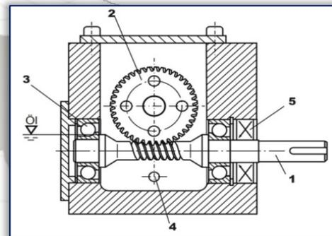
Figure 2b. Test transmission: 1 - worm shaft; 2 - worm gear; 3 - angular contact ball bearing; 4 - thermocouple; 5 - worm shaft seal
