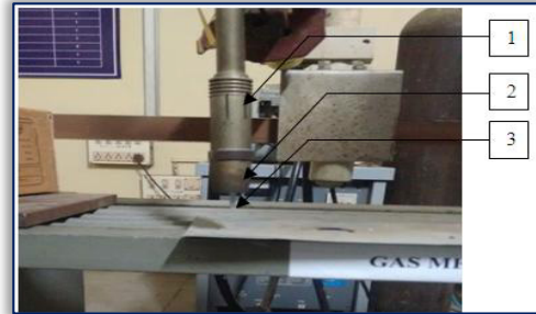
Figure 6. Setup of the SW - FCA Welding Process. 1 - SW-FCA welding torch; 2 - SW-FCA welding nozzle; 3 - Strip wire electrode.
