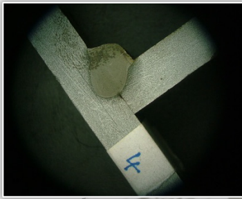
(b) Weld sample weld by SW-FCAW parallel to welding direction
