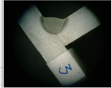
(d) Weld sample weld by FCA Welding
