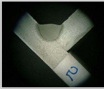
(a) Weld sample weld by SW-FCAW normal to the welding direction
