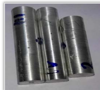
Figure 8. Specimen before Compressive Failure
