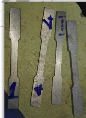
Figure 7. Tensile Specimens using EDM
